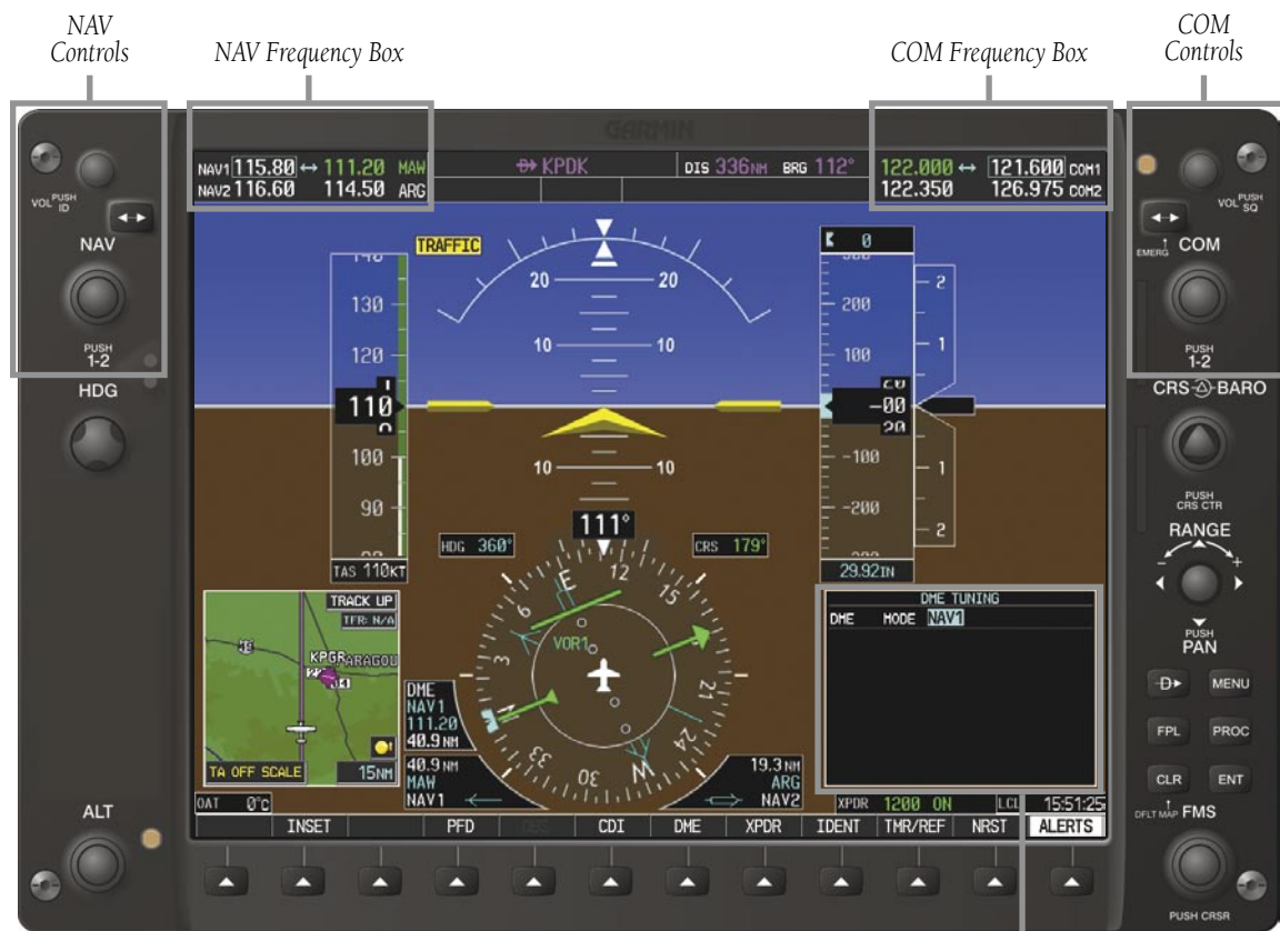
Figure 4-1 G1000 VHF NAV/COM Interface (PFD shown)
