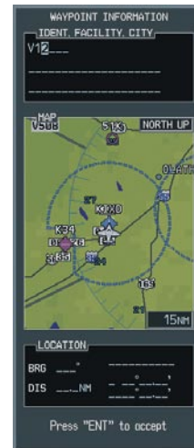
Figure 8-16 Enter Airway Identifier
