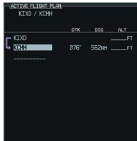
Figure 8-13 Airway Insertion Point
